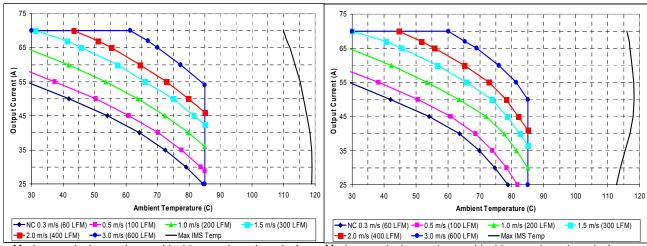
Maximum output current vs. ambient temperature at nominal input voltage for airflow rates natural convection (0.3m/s) to 3.0m/s with airflow from pin 3 to pin 1.
